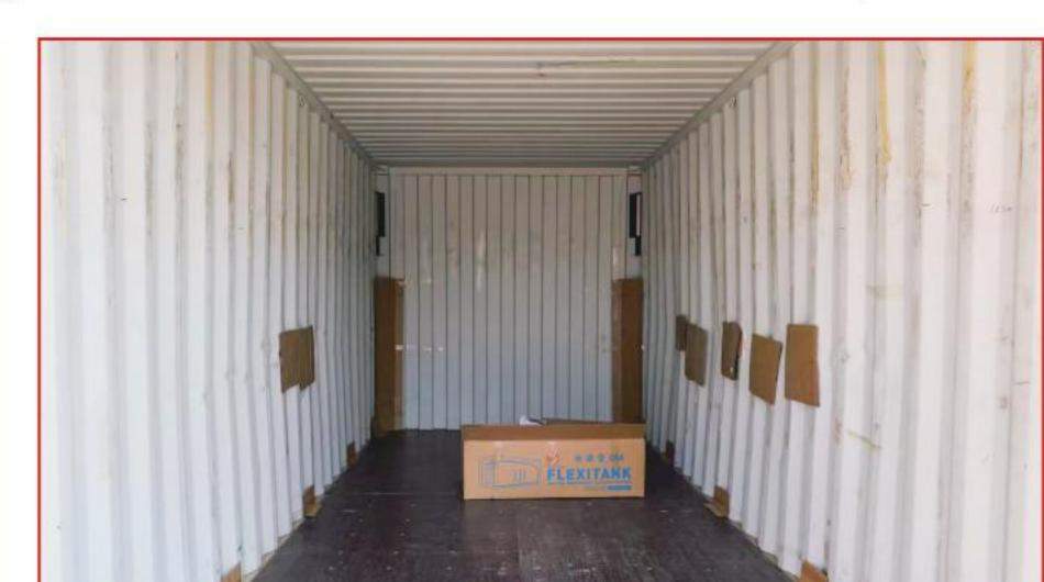
divide it into pieces with around 20cm side lengths. When there are hidden dangers such as welding spots and unevenness on the side walls and floor of the container, use the cut cardboard to protect the flexitank from potential damage.
